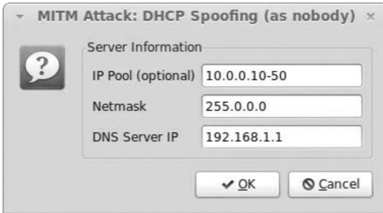
Figure 4-6: Configuring DHCP spoofing
