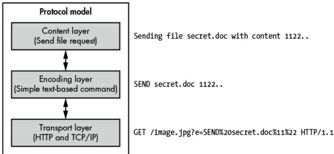
Figure 1-8: The conceptual model for a malware protocol using HTTP
