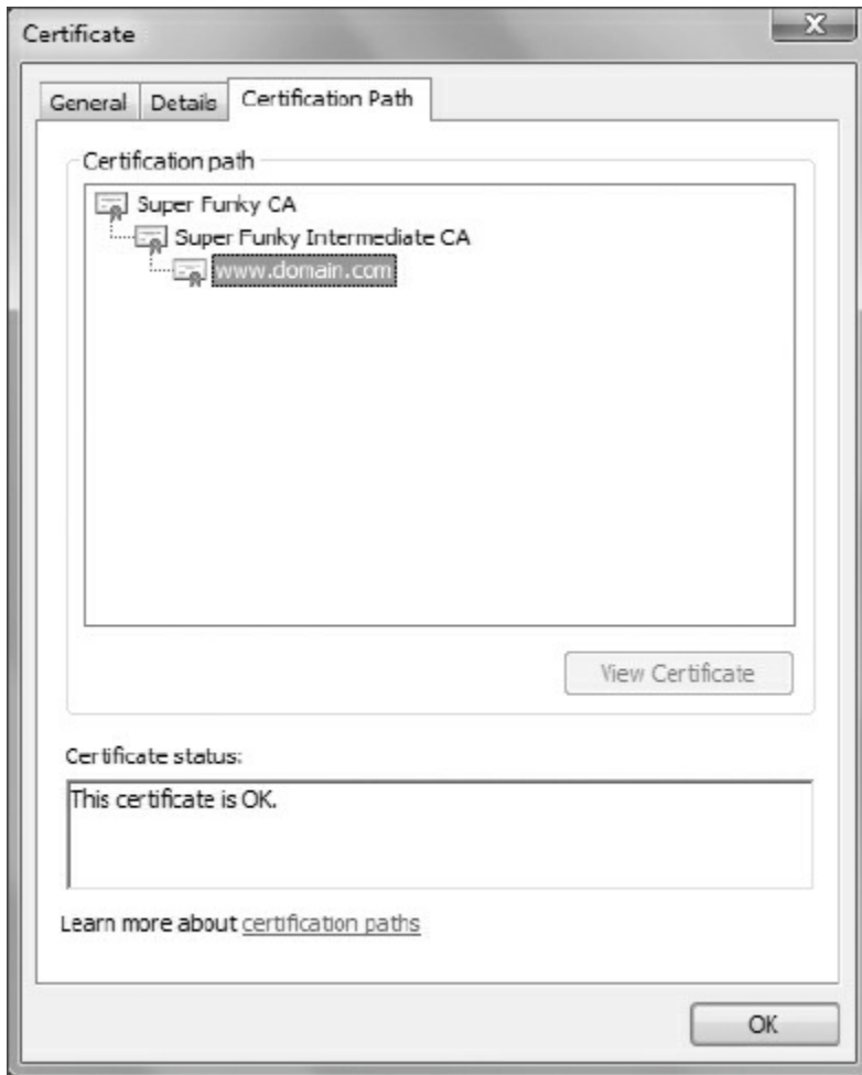
Figure 7-21: The chain of trust for www.domain.com
